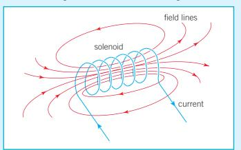
*Inside a solenoid* the magnetic field is *strong* and *uniform*, which means it has the same strength and direction at all points.
