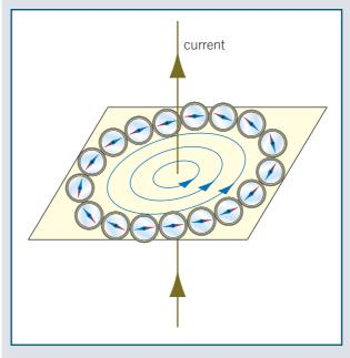
If the wire was gripped by someone's right hand so that the thumb pointed in the direction of the current, the fingers would curl in the direction of the magnetic field.
