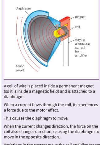
Variations in the current make the coil and diaphragm vibrate.
