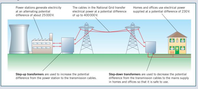
By making the grid potential difference much higher, a smaller current is needed to transfer the same power. Therefore, the National Grid is an efficient way to transfer power due to less heating loss in the wire.
